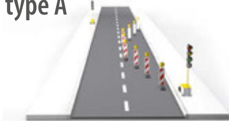
Fixed time control
